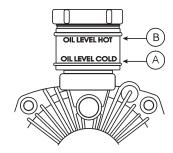
Figure 9. Transmission Reservoir
